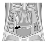
The vehicle has an Electric Parking Brake (EPB). The switch for the EPB is in the center console. The EPB can always be activated, even if the ignition is OFF. To avoid draining the battery, do not cycle the EPB too often without the engine running. The EPB can be left applied while the vehicle is parked.
